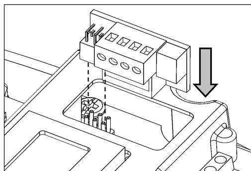
**CAUTION:** The auxiliary I/O board is separated from the main network through a "principal" insulation type (basic insulation according to EN 60730-1). Any circuit connected to this terminal will acquire the same level of insulation with respect to the mains power supply. For this reason the connections must be carried out with a cable type that guarantees the additional insulation.
