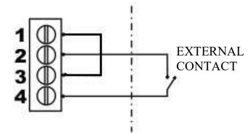
**ATTENTION:** incorrect wiring of the auxiliary contact may cause the low voltage circuit to short circuit with consequent blowing of the fuse! Carry out the connection with particular care.
