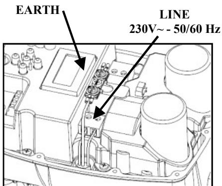
The device has a single-phase 230 Volt 50/60Hz power line.
