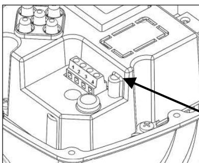
Sirio is fitted with a special connector for an auxiliary contact so that additional functions can be exploited by interfacing the device with external equipment. The function of the auxiliary contact depends on the setting of the “Auxiliary Contact” parameter described in the paragraph on programming. The three operational modes, relevant functions and connection methods are described below.
